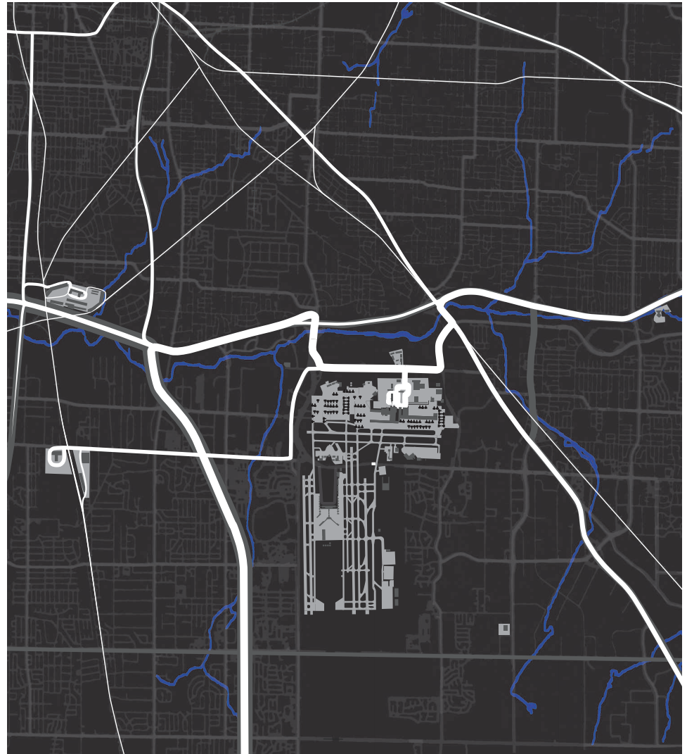
Above: Aerial Diagram of Memphis International Airport, illustrating hierarchy of ground shipping routes by volume. Bold lines indicate heavily traffice primary routes along interstates and rail, while thin lines represent secondary regional routes. Gray lines represent local roads. (Source: Shelby County GIS).
